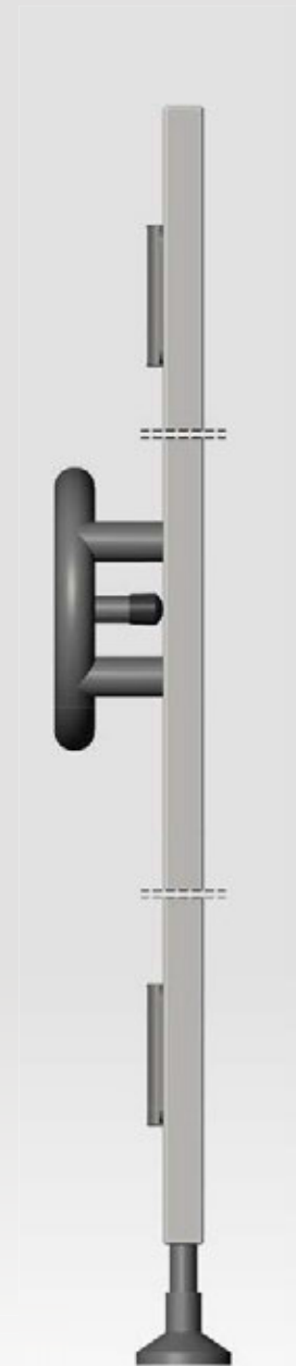
Aluminium tube with height-adjustable nylon rosette
